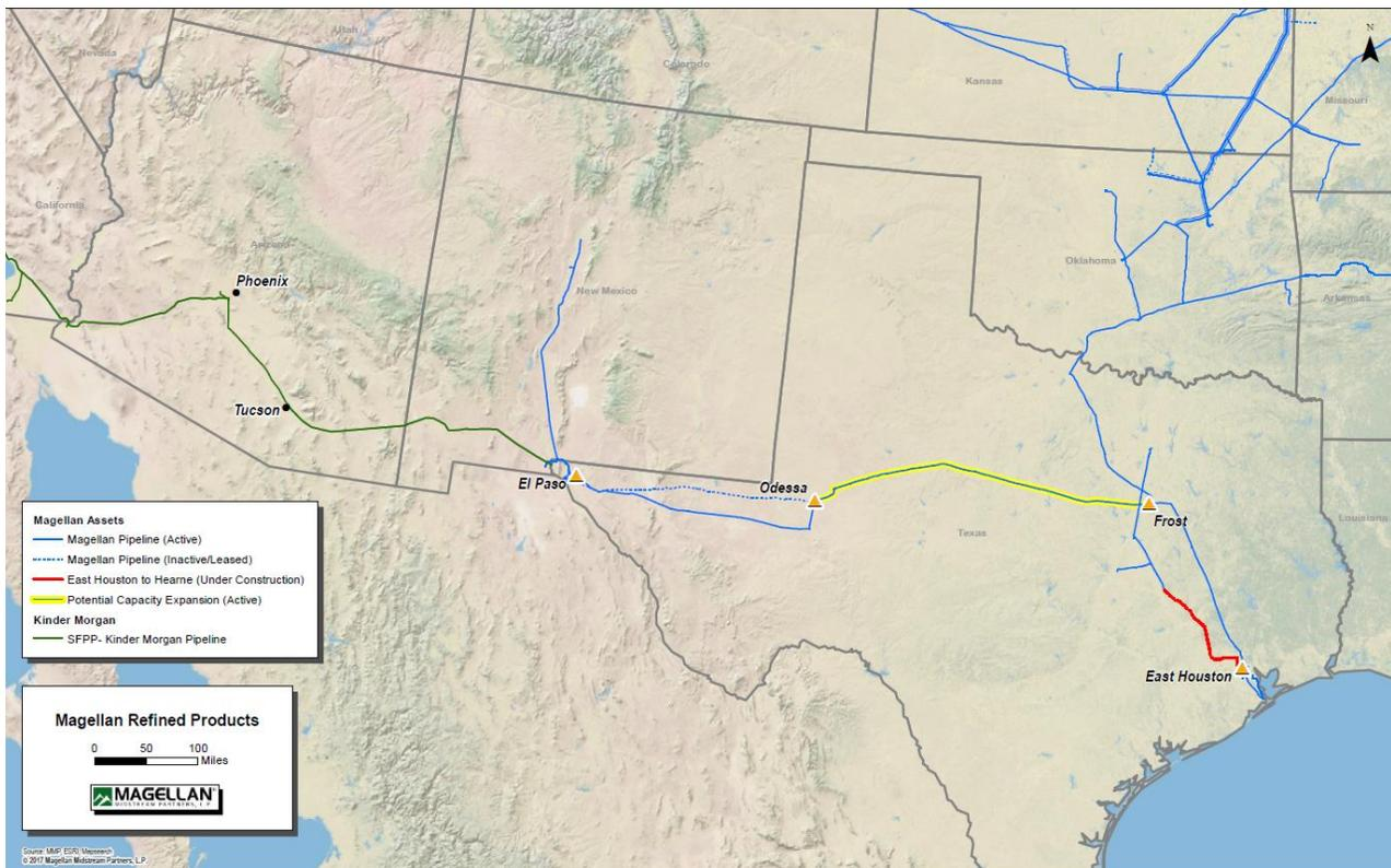
The current capacity on Magellan's West Leg is approximately 100,000 barrels per day ("BPD") in refined products service. Once the expansion is completed, the capacity on the West Leg would increase to approximately 140,000 barrels per day.
